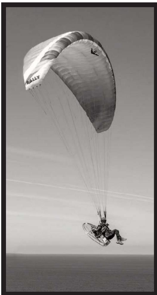
The **RALLY** has a brake of medium hardness (from 1.5 to 3 kg of effort, for most of the manoeuvres) the stall is outside the brake travel, and to access this configuration (not recommended in any type of paraglider) It takes more than 9 kg of effort and take it a couple wraps in the brake line.
