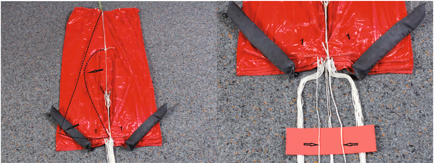
15. Arrange panel 1 (corner panel) and place a packing weight on the hem.
