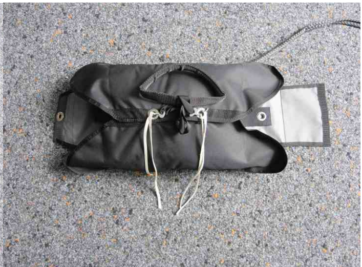
2. Close the two lateral flaps of the outercontainer with two packing-cords and closed it with the pins of the handle provisionally.
