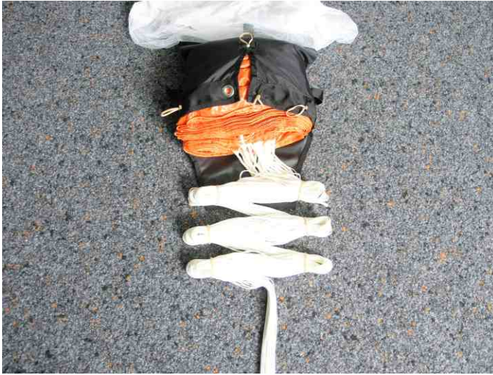
13. Bundle the lines in 3x3 "8-shapes". Do not bundle the last 60cm of the lines.
