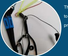
The first part needs to run through the ring that is closer to you accounting that you haven't turned the risers in the process.
