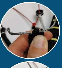
You can now detach the old line easily. You will find the connection in the socket where you hold the BC system normally while flying. Detach the line completly. NEVER TURN THE RISERS ON THE TABLE ONCE YOU DO THIS.
