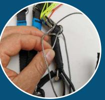
From the Tylaskaa ring, we return back with the line to the ring that is pointed away from us. Run the line from the outside of the riser towards inside moving down to the blue socket.
