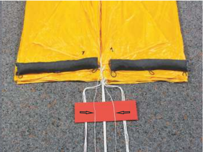
20. Check line 1 and 2 (arrows) and the center lines are not crossed and running free.
