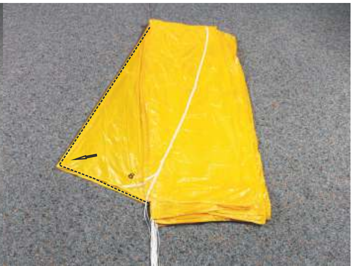
12. Place panel 9 (Ultra Cross 100/125) centered to the the floor and arrange panel 8 to the side. Ultra Cross 75: panel 7/6, Ultra Cross 150: panel 11/10, Ultra Cross 210: panel 13/12
