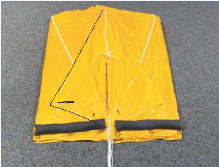
19. Arrange panel 1 (corner panel).
