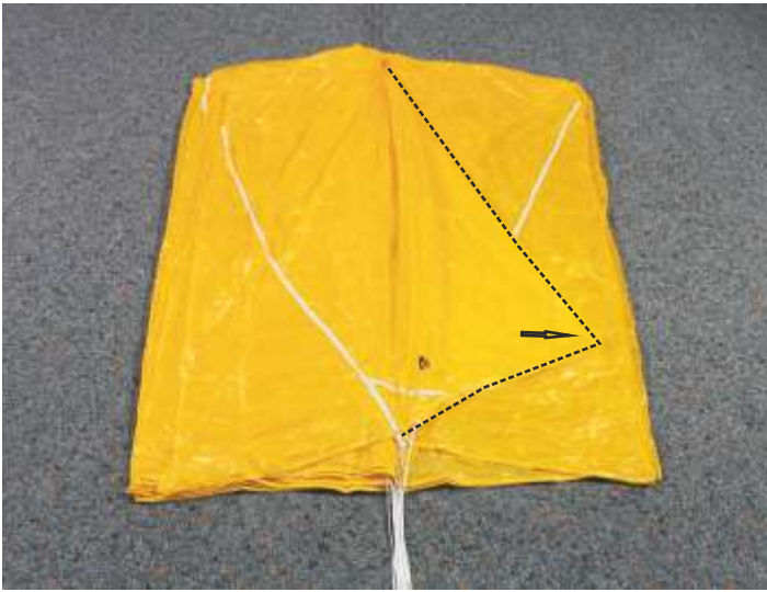
7. Arrange panel 4 (Ultra Cross 100/125). Ultra Cross 75: panel 3, Ultra Cross 150: panel 5, Ultra Cross 210: panel 6
