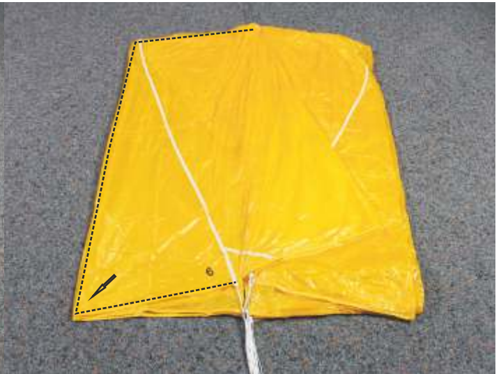
14. Arrange panel 6 (Ultra Cross 100/125). Ultra Cross 75: not applicable Ultra Cross 150: panels 8,7, Ultra Cross 210: panels 10,9,8
