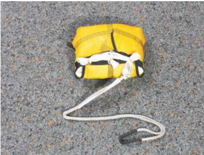
28. Close the deployment bag with the lines. First in the middle then the sides.
