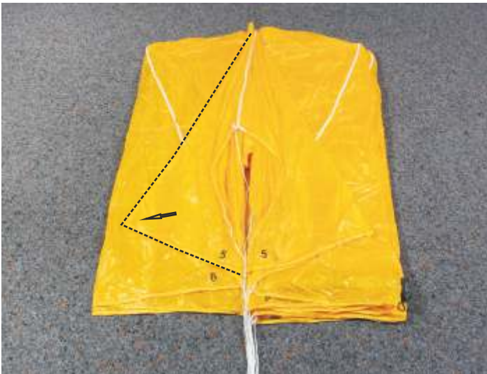
15. Arrange panel 5 (Ultra Cross 100/125) (corner panel). Ultra Cross 75: panel 4, Ultra Cross 150: panel 6, Ultra Cross 210: panel 7
