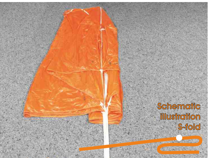
24. Fold right side S-shaped. (Step 1)
