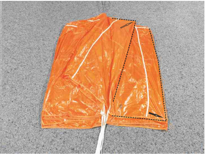
8. Arrange panel 6 and upper part of panel 5 to the side. (Evo Cross 160: panel 7, upper part of panel 6)
