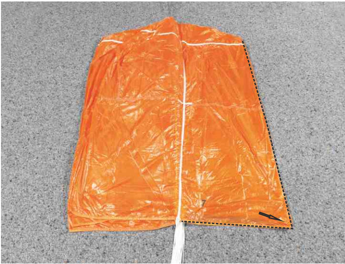
7. Arrange panel 7. (Evo Cross 160: panel 9/8)
