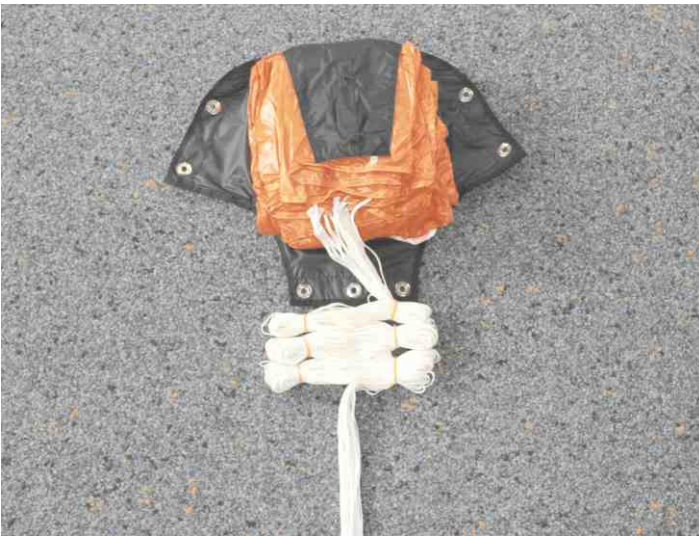
29 b. Bundle the lines in 3x3 "8-shaped" hanks. Do not bundle the last 70 cm of lines.
