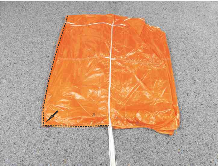
21. Arrange panel 3. (Evo Cross 160: panel 4/3)
