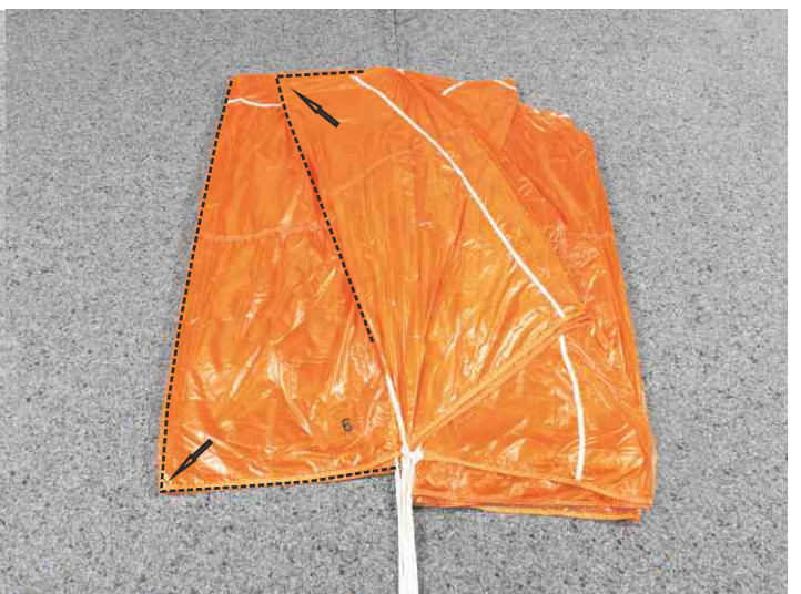
18. Arrange panel 6 and upper part of panel 5 to the side. (Evo Cross 160: panel 7, upper part of panel 6)
