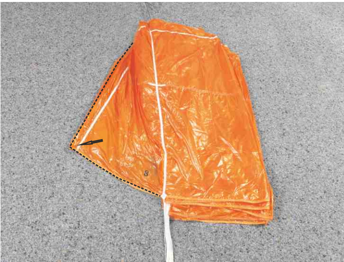
15. Place panel 9 (Evo Cross 160: panel 11) centered to the the floor and arrange panel 8 (Evo Cross 160: panel 10) to the side.
