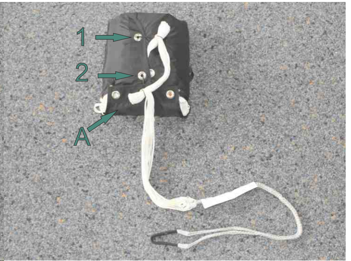
30 b. Close the deployment bag with the lines. First the long side. 1) then 2). No 2) is to be closed with the middle grommet of the remaining flap A).
