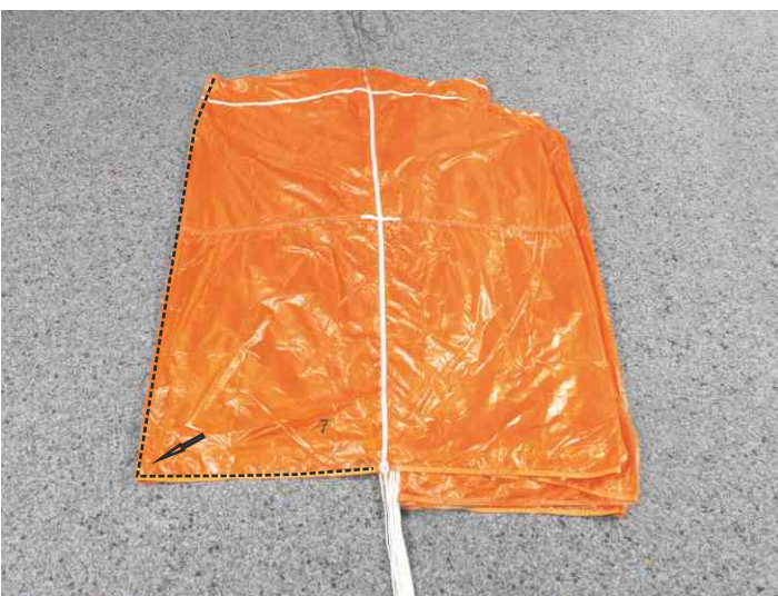
17. Arrange panel 7. (Evo Cross 160: panel 9/8)
