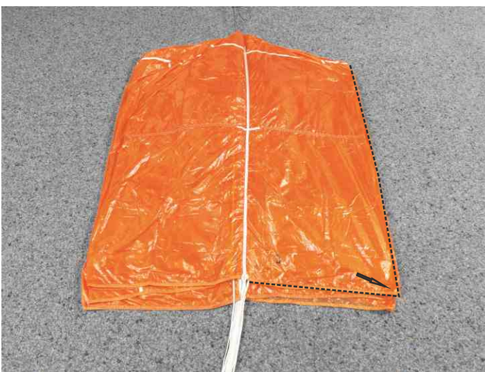
11. Arrange panel 3. (Evo Cross 160: panel 4/3)
