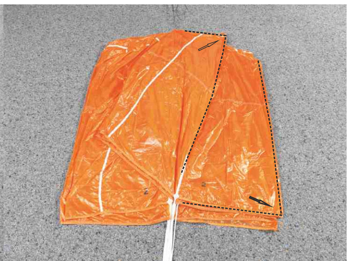
12. Arrange panel 2 and upper part of panel 1 to the side.
