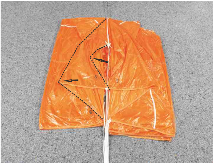
19. Arrange panel 5 (corner panel) (Evo Cross 160:panel 6)
