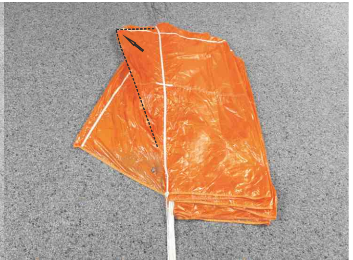
16. Arrange the upper part of panel 8 (Evo Cross 160: panel 10) to the side.
