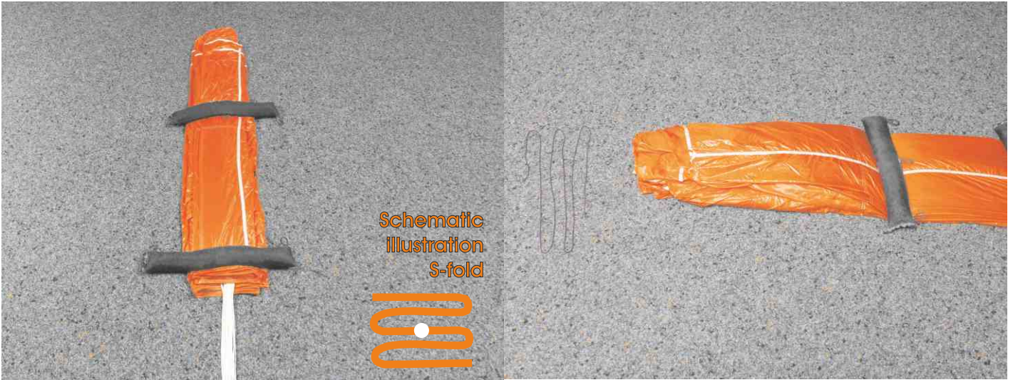
25. Fold left side S-shaped. (Step 2)
