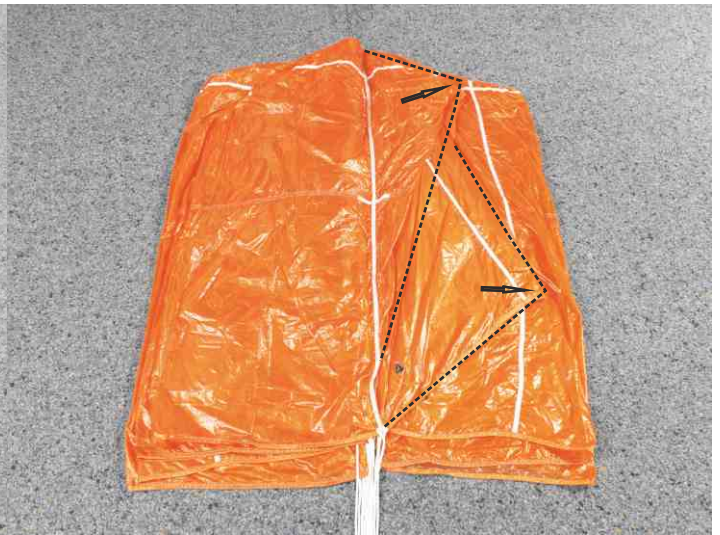
10. Arrange panel 4 and upper part to the side. (Evo Cross 160: panel 5)
