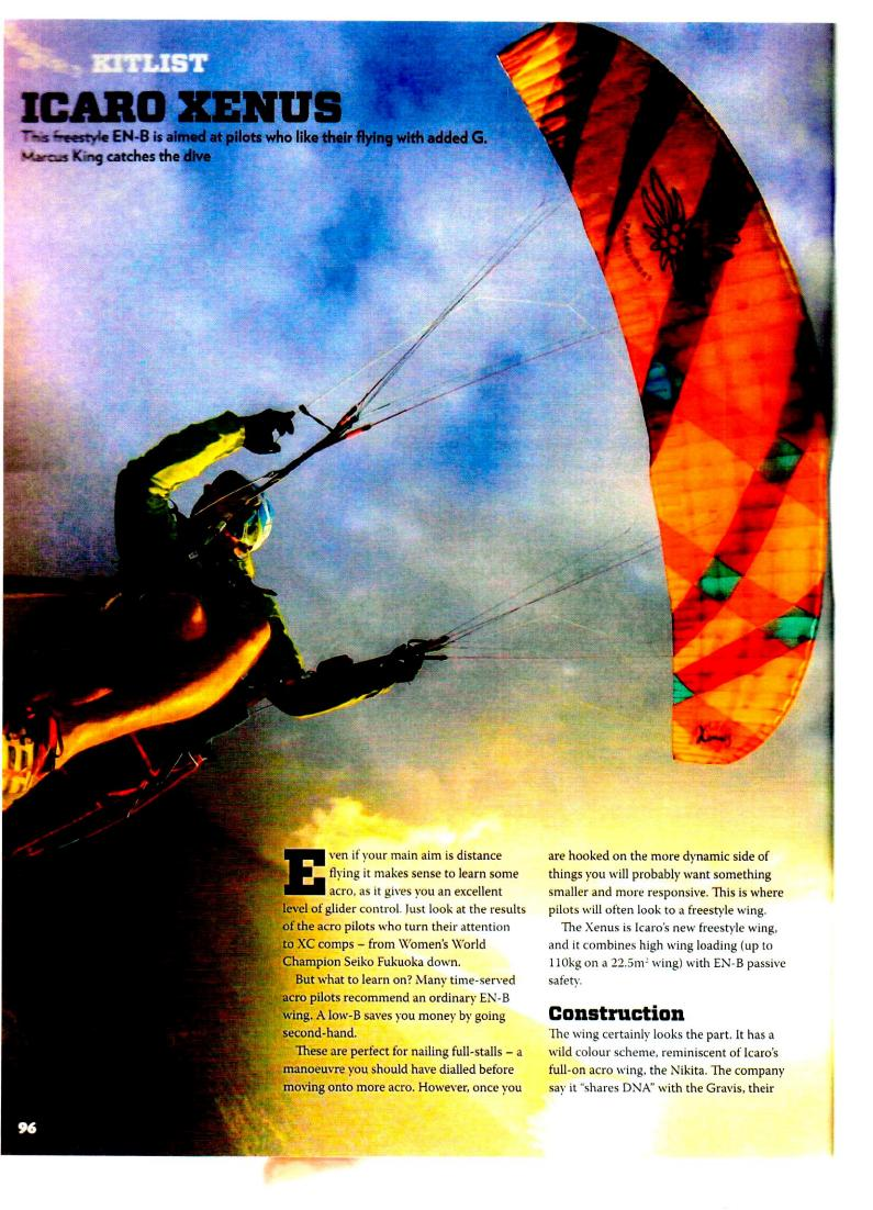
mid-to-high EN-B wing. It has the same 40 cells, a sharknose up front and mini-ribs on the trailing edge.
