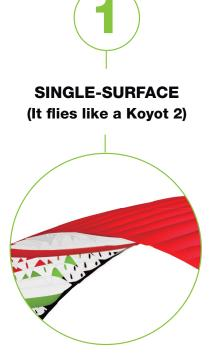
A single-surface glider to ensure the wing is light and easy to fly without compromising on performance.
