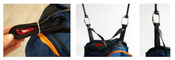
The two connections should be made using screw-lock snap-hooks with a breaking strength of at least 1,400 kg. It is important to make sure that the bridle is long enough to position the reserve parachute inside the harness pocket and that there is sufficient room to take the parachute out of the pocket without causing the reserve parachute deployment bag itself to open during extraction.
