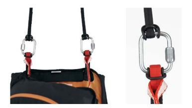
The two connections should be made using screw-lock snap-hooks with a breaking strength of at least 1,400 kg. It is important to make sure that the bridle is long enough to position the reserve parachute inside the harness pocket and that there is sufficient room to take the parachute out of the pocket without causing the reserve parachute deployment bag itself to open during extraction.
