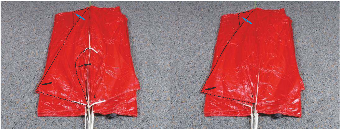
11. Arrange panel 6 (corner panel). Pull out the upper part of the canopy (blue arrow).
