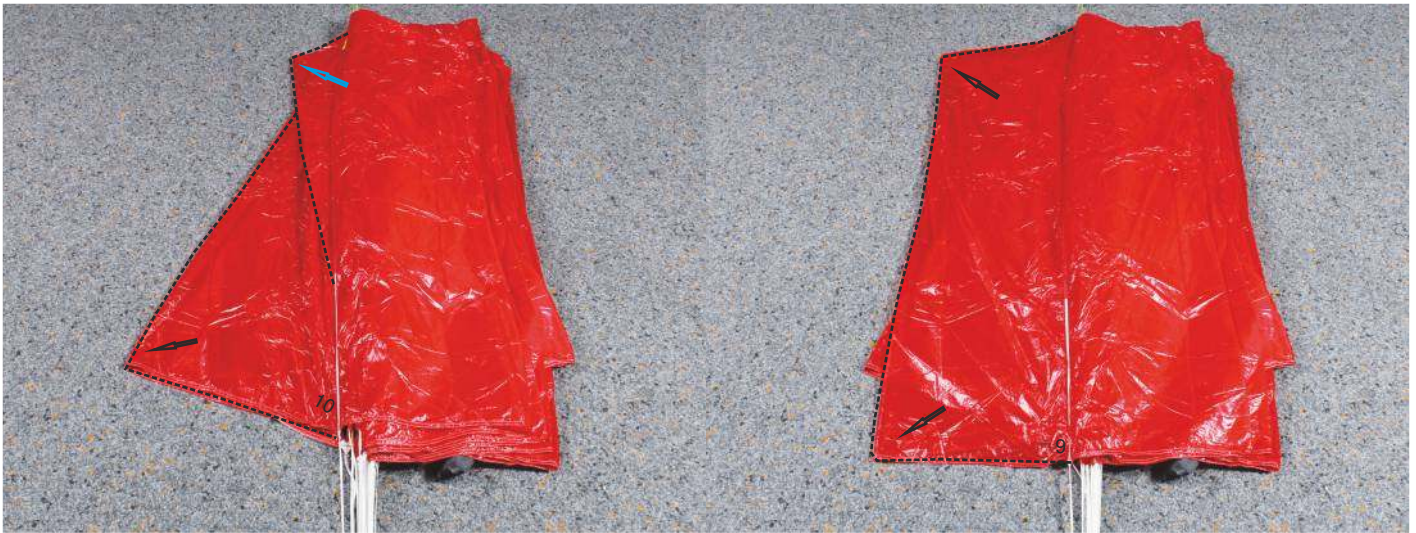
9. Place panel 11 centred on the floor, pull panel 10 out to the side, as well as the upper part (blue arrow).
