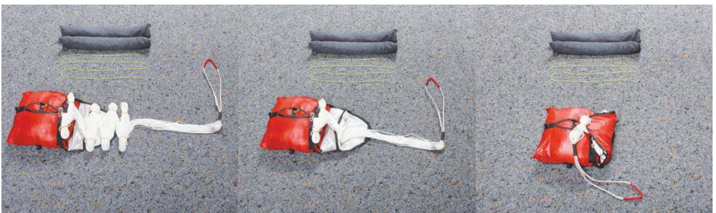
19. Close the container. First the middle, then the outside. Bundle the lines in 3 x 3 "8-shaped" hanks. Do not bundle the last 60 cm of lines.
