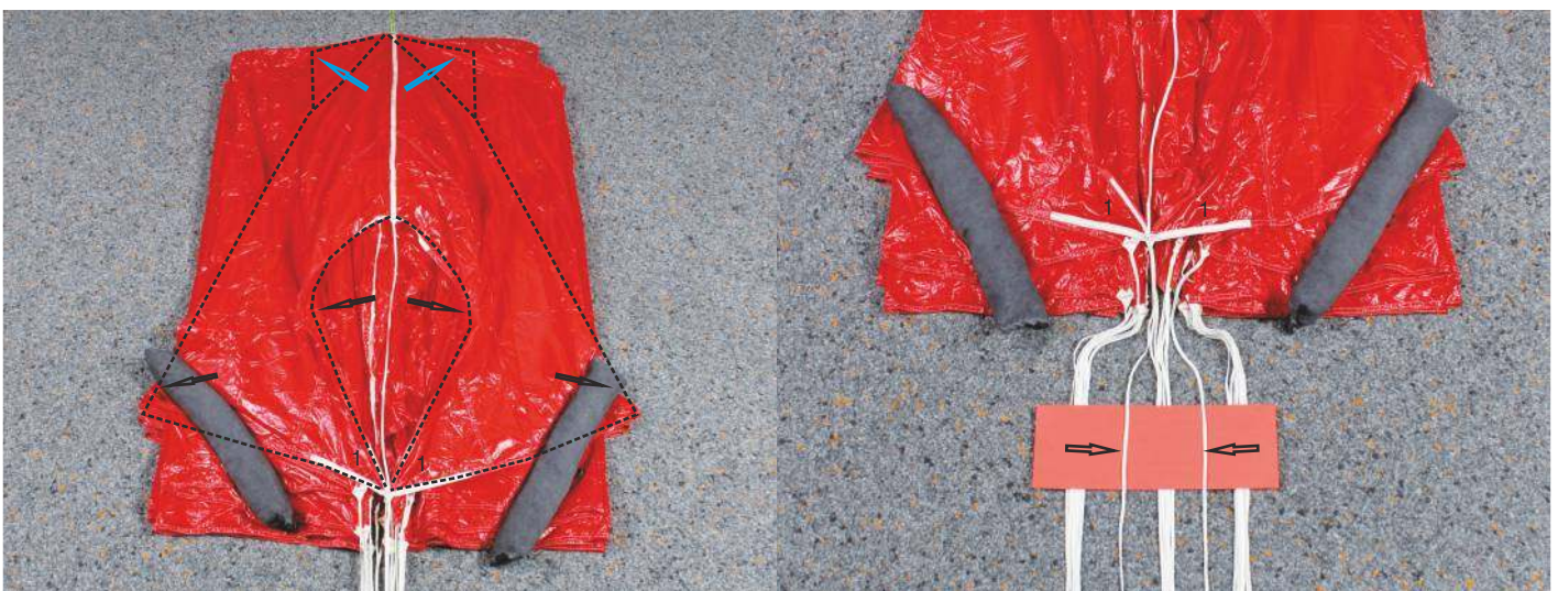
13. Arrange panel 1 (corner panel) and weigh down the hem with a weight.
