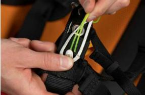
Take care that both ends of the overlap of the strap come out of the loop and are visible; also check that the knot is properly tightened. Specifically, take care that the overlap does not get caught on the white loop.
