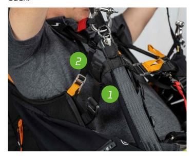
In detail, adjustment 1 varies the angle between the legs and the back (seating depth), distributing the loads between the seat and the lumbar, thereby providing the pilot with greater comfort. The main adjustment that allows you to select the inclination of the torso with respect to the vertical flight axis is No.2 for back adjustment.
