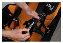
CAUTION: the white loop closing the three rings must be fixed where the seam is and thus where the strap overlaps.
