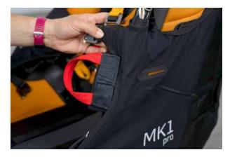
When tensioned, it activates the "3-ring" release and lets the pilot quickly separate from the paraglider wing and then open the reserve BASE without it interfering with the main glider.
