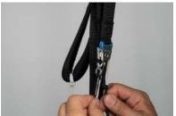
If the speed-bar cord is too short, it could cause a constant force on the speed-system during flight, so that it is unintentionally engaged at all times in flight. It is safer to take off with the speed-bar a little longer and to shorten it gradually during subsequent flights. Remember that all adjustments have to be performed symmetrically, on both sides.
