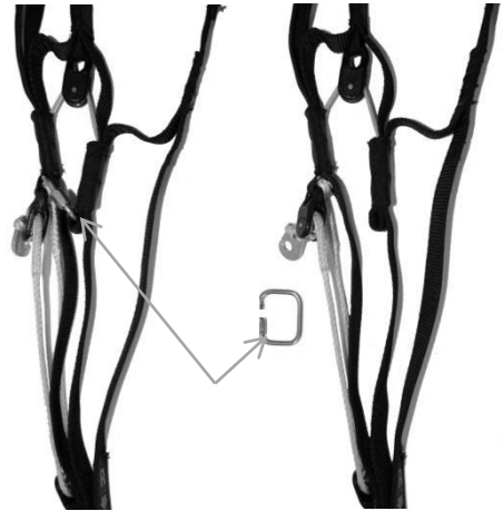
Fig. 13 MITO riser with and without speed limiter
