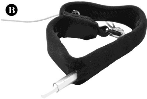
B To remove the stiffeners, turn the Multigrip brake handle inside out and push the two small rods out through the opening
