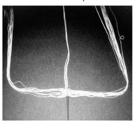
Please make sure that the middle lines are in the middle and the other lines to the side. There must not be any tangles or knots in the lines.
