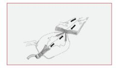
STEP 2: Make sure the parachute is completely disentangled and that both the lower line and the upper of the reef knot run freely from the risers to the canopy.
