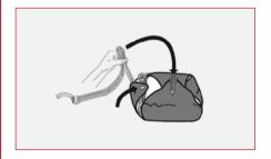
STEP 16: Close the fourth flap and put a coil of lines (about 4 cm) through the loop of the flap with the rubber fitting in order to hold the container closed.
