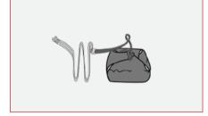
STEP 17: Coil the remaining lines on the outside of the container.
