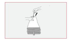
STEP 11: Squeeze the air out of the canopy then REMOVE THE TIE WHICH HOLDS THE FOLDING LOOPS TOGETHER. (See inventory list).
