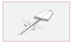
STEP 9: Check both lower and both upper lines to make sure that they run freely from the canopy to the riser(s).
