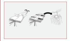
STEP 4: There are folding loops, nearly midway down the canopy where the panels were stitched. Pass a tie through these loops and stretch the parachute out.
