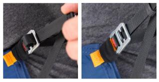
Our harness is supplied with the adjustment locked. To change the setting, you must first remove the strap from the lock, then you can adjust the inclination of the torso to make it more vertical by pulling the strap forward, or more reclined by pulling the light grey strap in the opposite direction.
