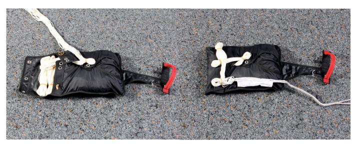
4. Close the deployment bag with the lines. First the right flap with the upper and lower flap. Depending of the rescue system size the inner or outer grommets can be used to adjust the deployment bag volume.
