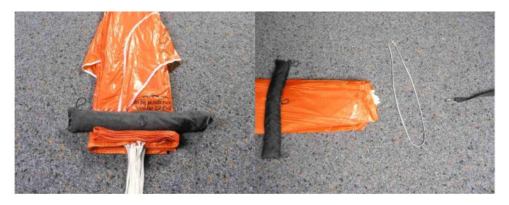
1. Fold the parachute like a "S" on the width of the container, pull out the Ram-Air-pockets a little bit to the side (if the parachute is equipped with Ram-Air-pockets).
