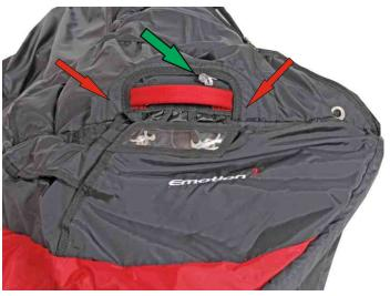
6. Remove all packing cords! Close pin cover and place the handle in the neoprene pockets (red arrow), secure handle with a 2 daN seal threat (green arrow).
