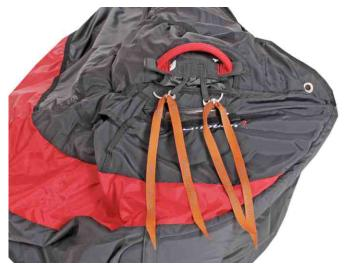
5. Close lower container flap with packing cords. Put the pins through the loops.
