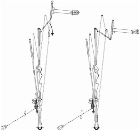
Fig. 7 Stabilizing by C-bridge
