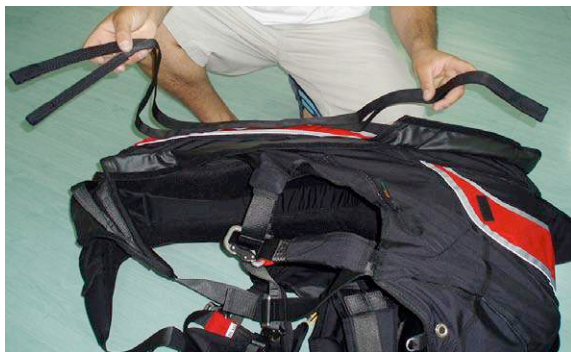
Preparation of the second V-line: Pull the end with the two loops upward towards the shoulder strap. The end with one loop leads to the reserve.
