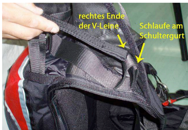
picture of correct placement of the V-line, showing the placement of the loop to be connected with the shoulder strap
