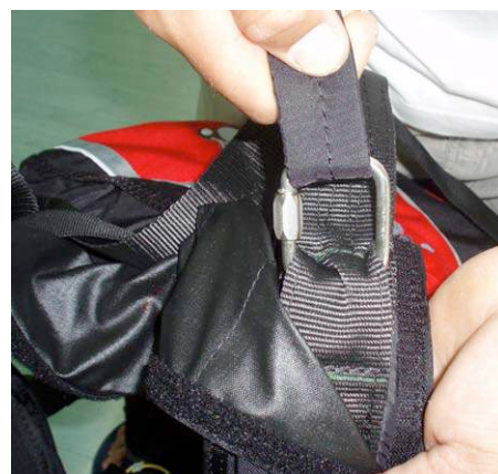
Connection of both ends of the V-line and shoulder strap with metal connection link
