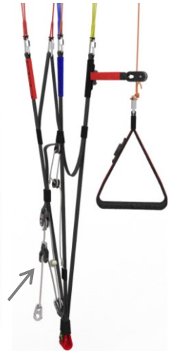
Fig. 4 MIURA RSe riser with speed limiter
