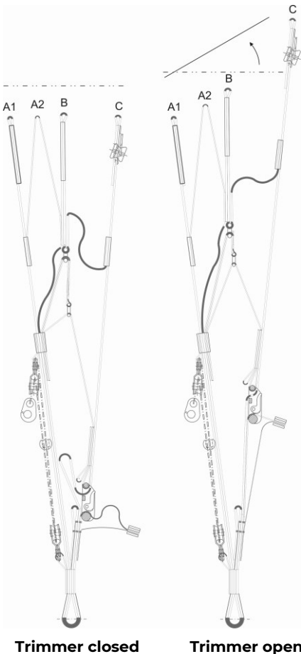
Fig. 14 How the trimmers work
