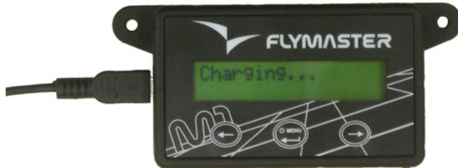
Figure 1: Battery charger connection
