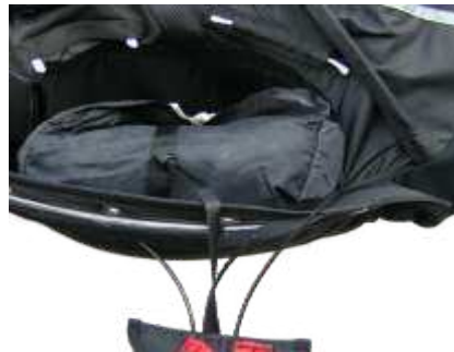
Put in the rescue-system container. The connected handle is showing to the seatboard and the container opening of the harness.
