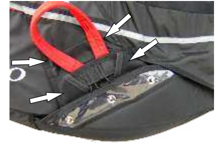
After closing the container, by putting in the pins, remove the packing cords and put the release-handle in the therefore assigned pockets
