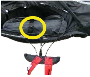
Fix the Harness Handle on the Rescue Container
