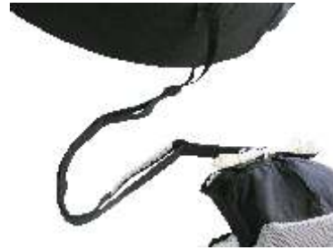
Connection between Rescue and Harness
