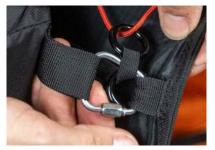
To install the soft links, follow the procedure as shown in the pictures below. Put the soft link first into the harness front loop behind the two rings held together with the elastic and then into the protection loop.
