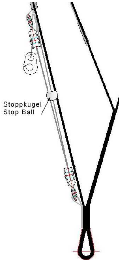
Fig. 7: Stop ball on the riser's speed bar line
