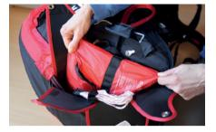
Insert the reserve with the handle attachment facing the seat board and the lines straight underneath.
