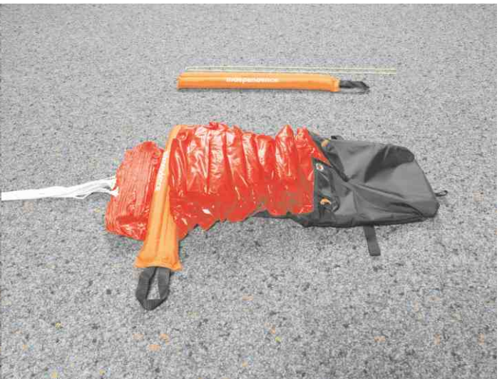
10. Put the upper part of the canopy into the inner container and fold the rest of the canopy in small S-shapes and place it in front of the inner container.
