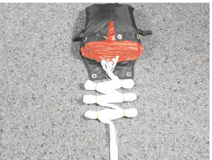
12. Bundle the lines in 3x3 "8-shapes". Do not bundle the last 50cm of the lines.
