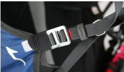
Fig. 6: Buckle blocked with mark showing standard position
