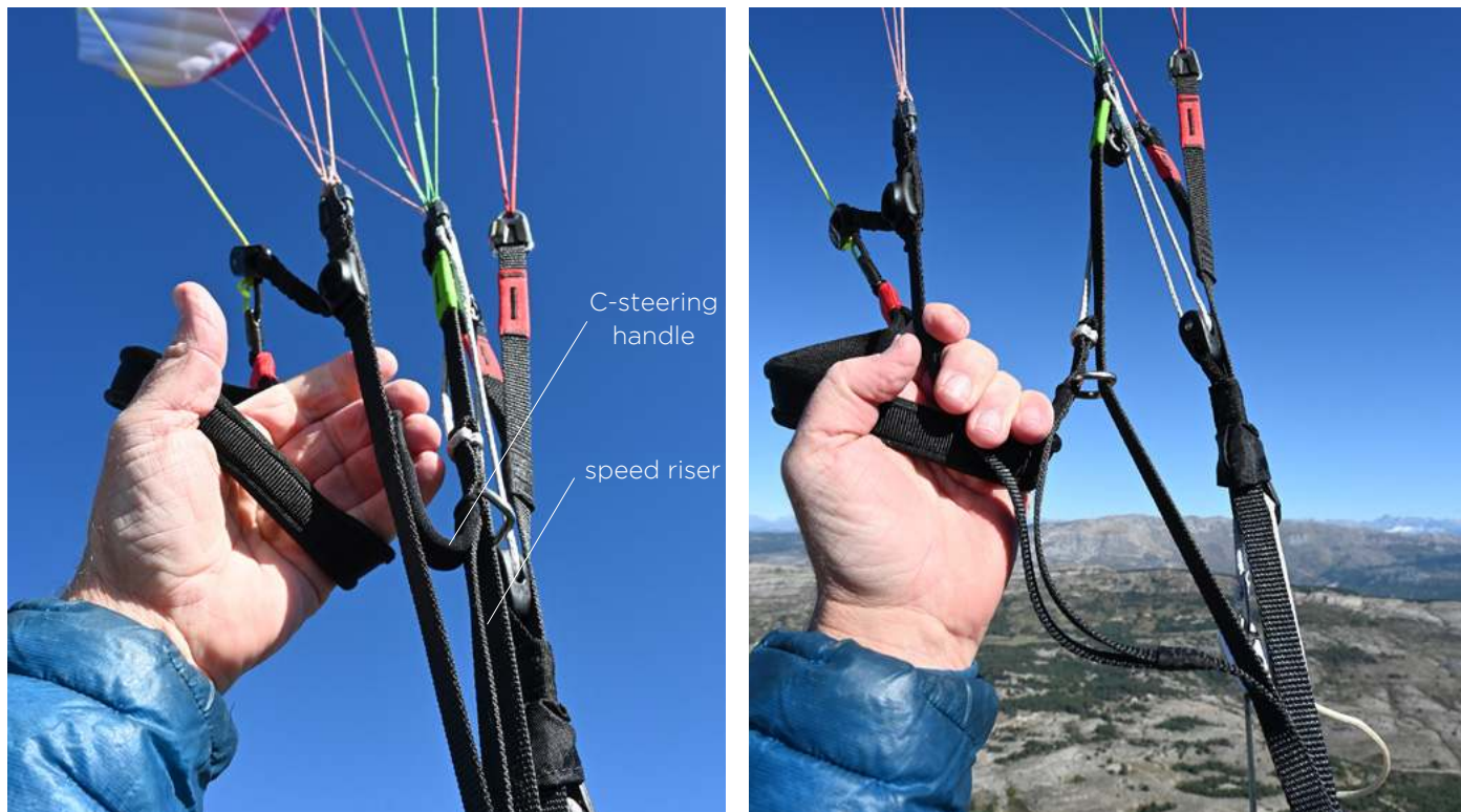
FIG. 1: Keeping the brake in your hand, grasp the C-steering handle with your fingers to apply pressure to the C's.
