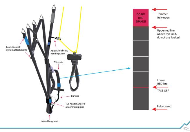
The updated risers feature long range trimmers with roller cam buckles; strong brake handle magnets; tip steering system (TST); fully adjustable brake pulley height settings; special brake handles; double launch assist system attachment points and coloured A risers for easy identification.
