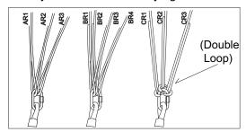
Factory delivered configuration with double loop on C-riser lines for trimming during aging
