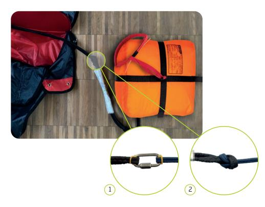
It is important to ensure that the connection is centered, both connecting lines that lead to the shoulder are of the same length. If the harness does not have an integrated attachment possibility for the reserve chute on the shoulder straps, then the reserve chute connecting line can also be attached to both main carabiners. For removal proceed in reverse order.
