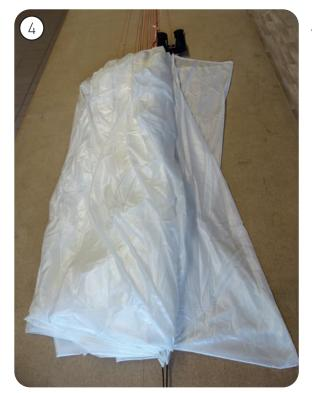
4. Pull the base from one line attachment point to the next along the seam to the side you are sorting and smooth the crossed panel. A line separator and a weight will help to secure the already sorted lines.
