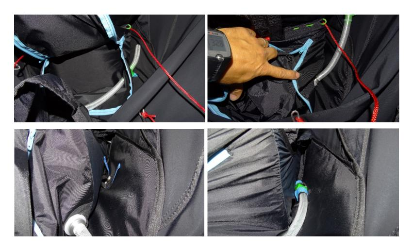
The ballast compartment is located beneath the seat. Open the zipper to access and insert the discharge tube into the hole on the right and install the ballast. Slide the tube into the sleeve on the side until it comes out of the other side. Lodge the tap in the hole and use the blue Velcro strap to secure the tube so that it remains in place.
