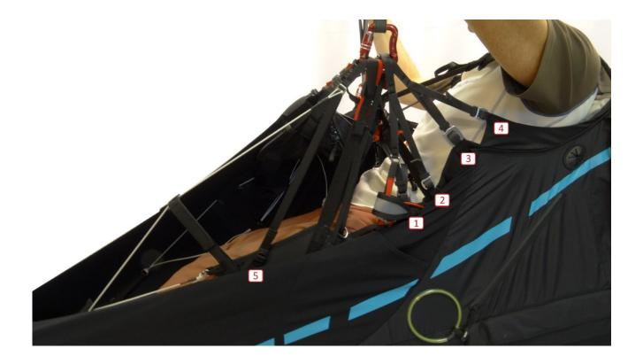
In the detailed photo, adjustment n° 1 changes the angle between thighs and back (seat depth), distributing load between seat and the lumbar area and thus improving pilot comfort.
