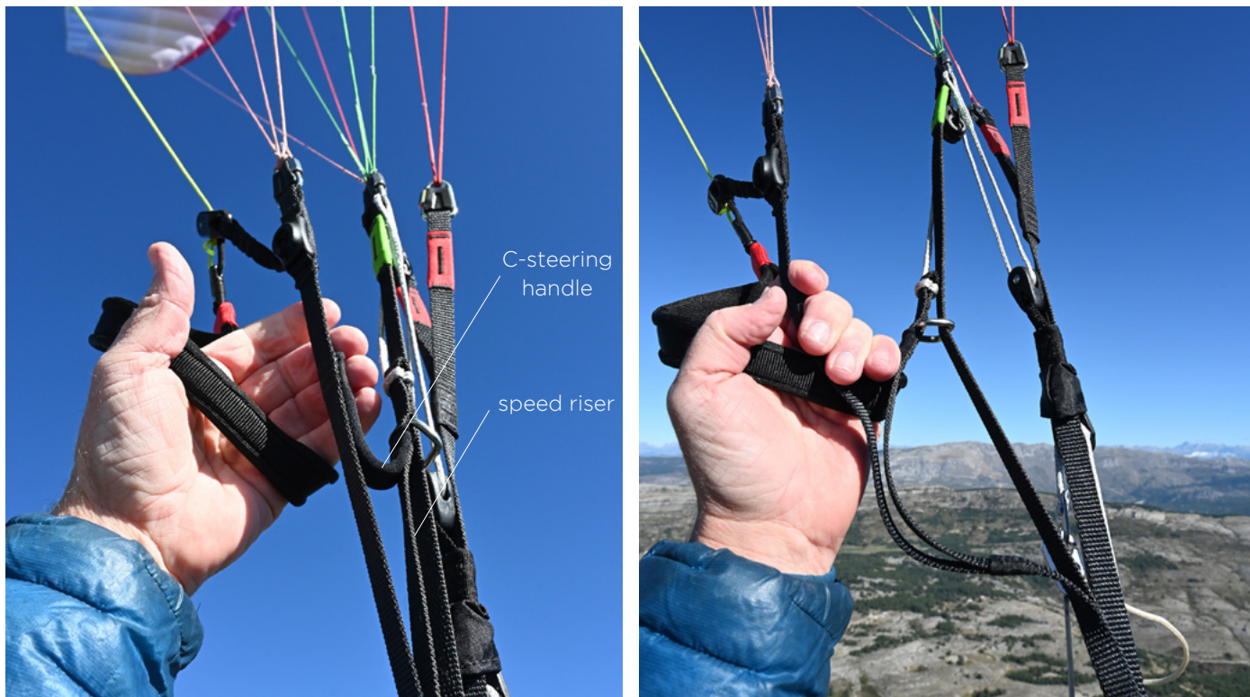
FIG. 1: Keeping the brake in your hand, grasp the C-steering handle with your fingers
