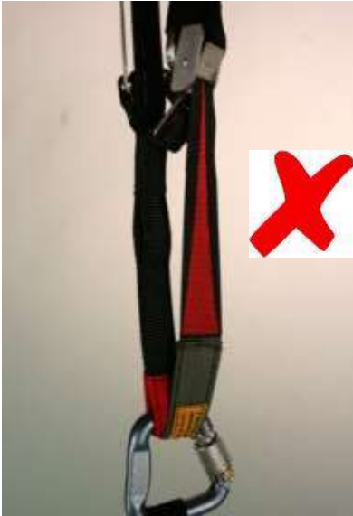
Fig. 11: Trimmer loop in the main carabiner
