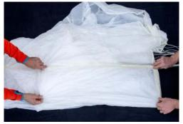
The last one is panel 1, which should be the top panel on the left side. Panels with slots are laid out as cone.
