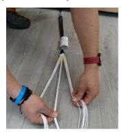
Check for the lines to run freely from the main riser loop connection to the canopy edge.
