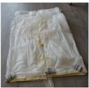
To help you pack the rescue system, use a short piece of old paraglider line and thread it through all the apex fixing loops. The fixing loops are sewn on the canopy.
