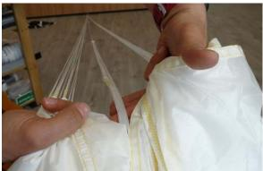
For easy control divide the lines in two sections with the same numbers of lines, the apex line must be placed in the middle.
