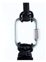
The two connections should be made using screw-lock karabiners with a breaking strength of at least 1,400 kg. In any case, it is important to verify that the length of the bridle is sufficient to position the reserve parachute inside the harness pocket, and that there is sufficient play to enable the parachute to be taken out of the pocket without causing the reserve parachute deployment bag itself to open during extraction.
