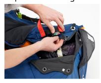
Introduce a thin rope (like paraglider line) into each elastic loop which you will use to help close the container. Insert the elastic loops into the smallest of the eyelets, marked with number 1.
