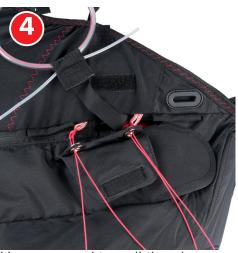
Use paracord to pull the closure loops through the secondary loops and metal eyelets
