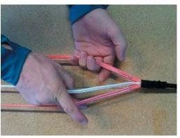
**13.** Now fold the reserve chute with an "S-fold" corresponding to your size and place the rescue container that the rescue flap with the rubber loop looks to the side (seen from the base).
