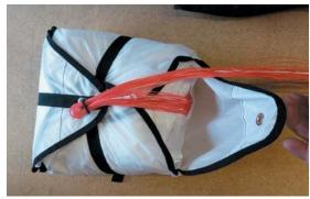
the line bundles in the shape of a figure-eight. Use siliconebased rubber rings to fix the line bundles.
