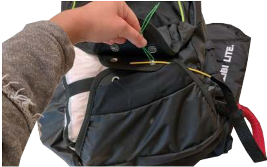
Push the yellow cable through the loop and gently pull the cord out.
