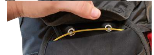
Push the loop through the upper grommet flap grommet and push the yellow cable through it ( loop ). Push the end of the yellow cable into the eyelet cut on the edge of the bottom flap.
